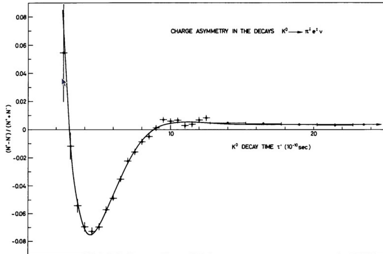
Fig. 1. The charge asymmetry as a function of the reconstructed decay time  $t'$  for the  $K_{e3}$  decays. The experimental data are compared to the best fit as indicated by the solid line.
