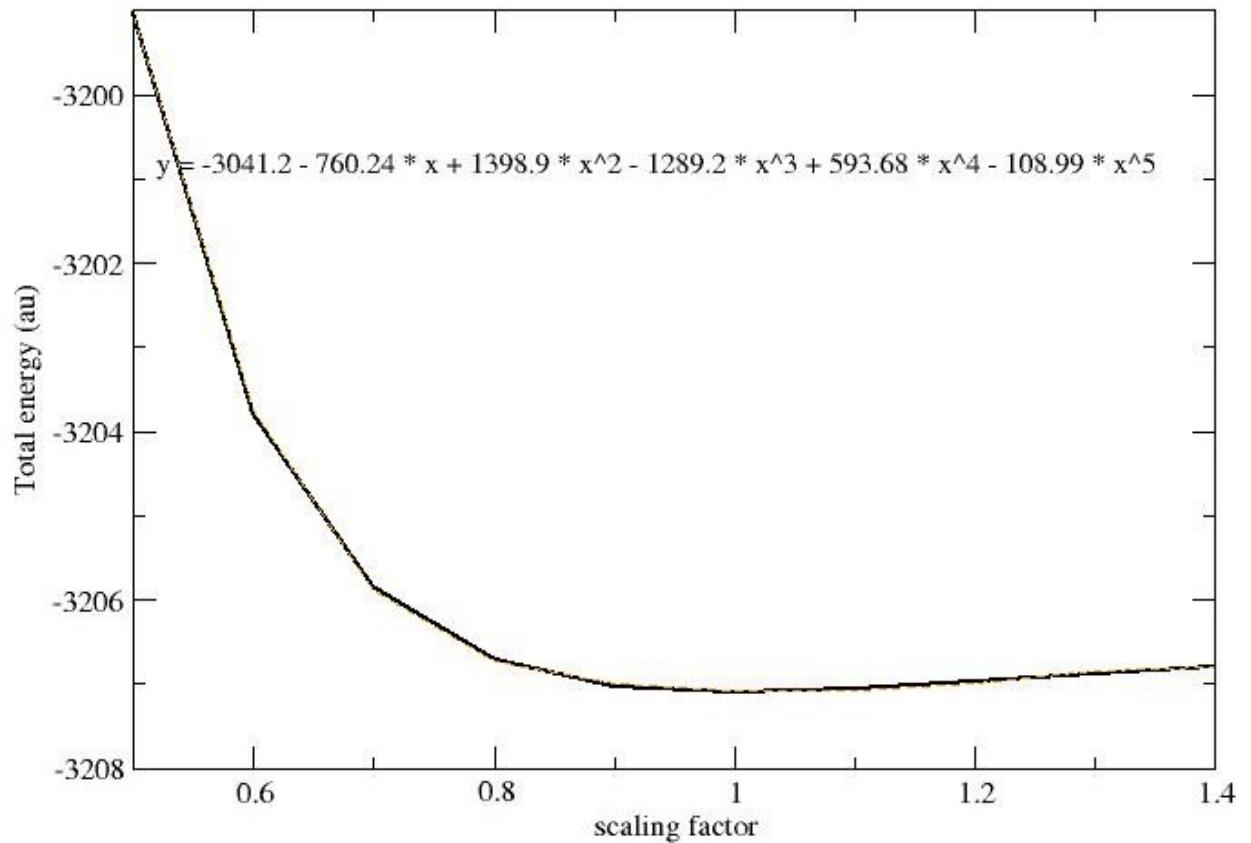
The total electronic energy shows a minimum near scaling factor 1.0.
