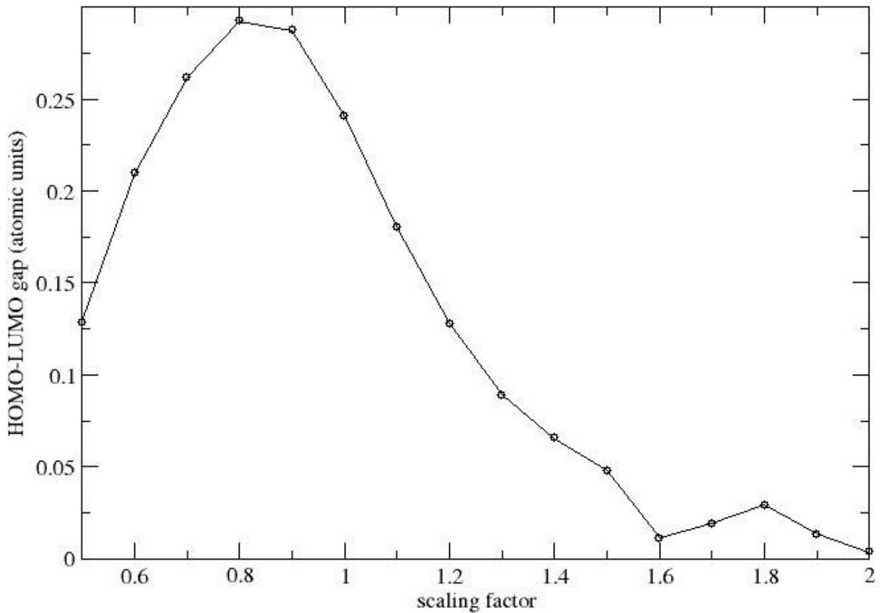
The bond stretching will inevitably lead to a breakdown of the SCF model. Indeed one observes that the HOMO-LUMO gap closes and the SCF did not converge beyond scaling factor 1.4. Further studies requires the calculation of  $E_{PV}$  using a method which can break bonds, e.g. MCSCF.
